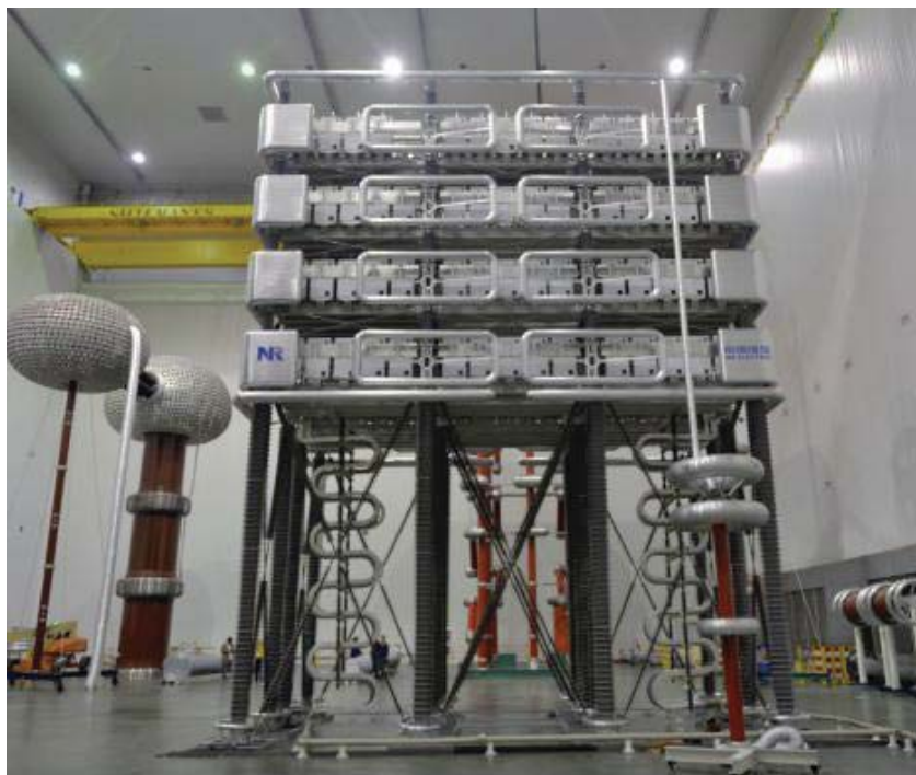
Figure 3 ±800kV/5000M VSC-HVDC Converter Valve
