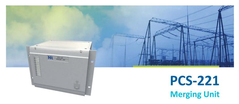
Merging units are used to sample AC analog values and transmit the sampled values(SV) to protection devices, bay control units(BCU) or electric meters through optical communication channels based on the IEC61850-9-2 protocol.
